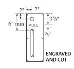
**Pull Positioning on** Plates Wider than 4" (Handing Required):
